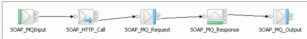
Figure 6-12 Sample message flow for synchronous interaction pattern
